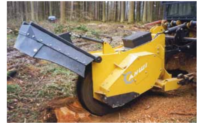
SF1000: The auxiliary attachment unit for the AHWI RT400 crawler tractor with a grinding depth of 35 cm max.
