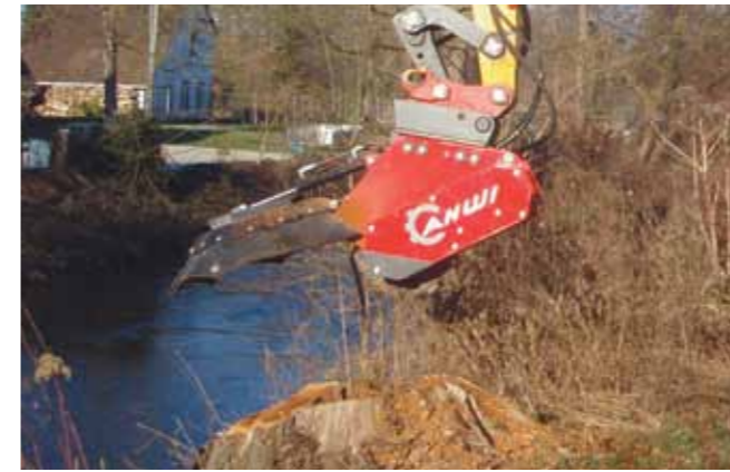
SF600H: For precision stump grinding in poorly accessible locations.
